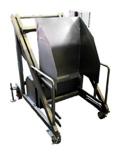
The hydraulic lift is designed for lifting and turning cutter carts with a volume of 100 liters.
